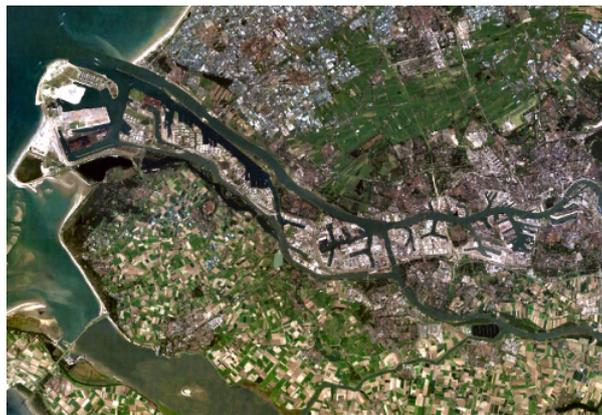
"Port of Rotterdam. Europe's largest port today in terms of traffic, the spatial development of the Port of Rotterdam was carried out using the construction of artificial embankments in the sea. The quality of its navigable network provides it with axes of penetration toward Central Europe. Source: Wikimedia Commons
