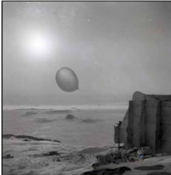
Launch of a ballon-sonde from the French Antarctic research station Dumont d'Urville during the International Geophysical Year in 1957. Expéditions polaires françaises, Fonds antarctique. Source : Archipôles .
